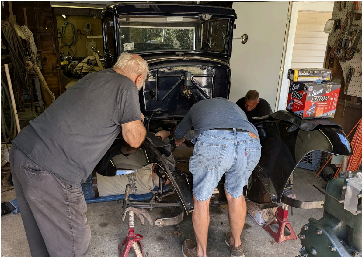
Installing the rebuilt torque tube!
