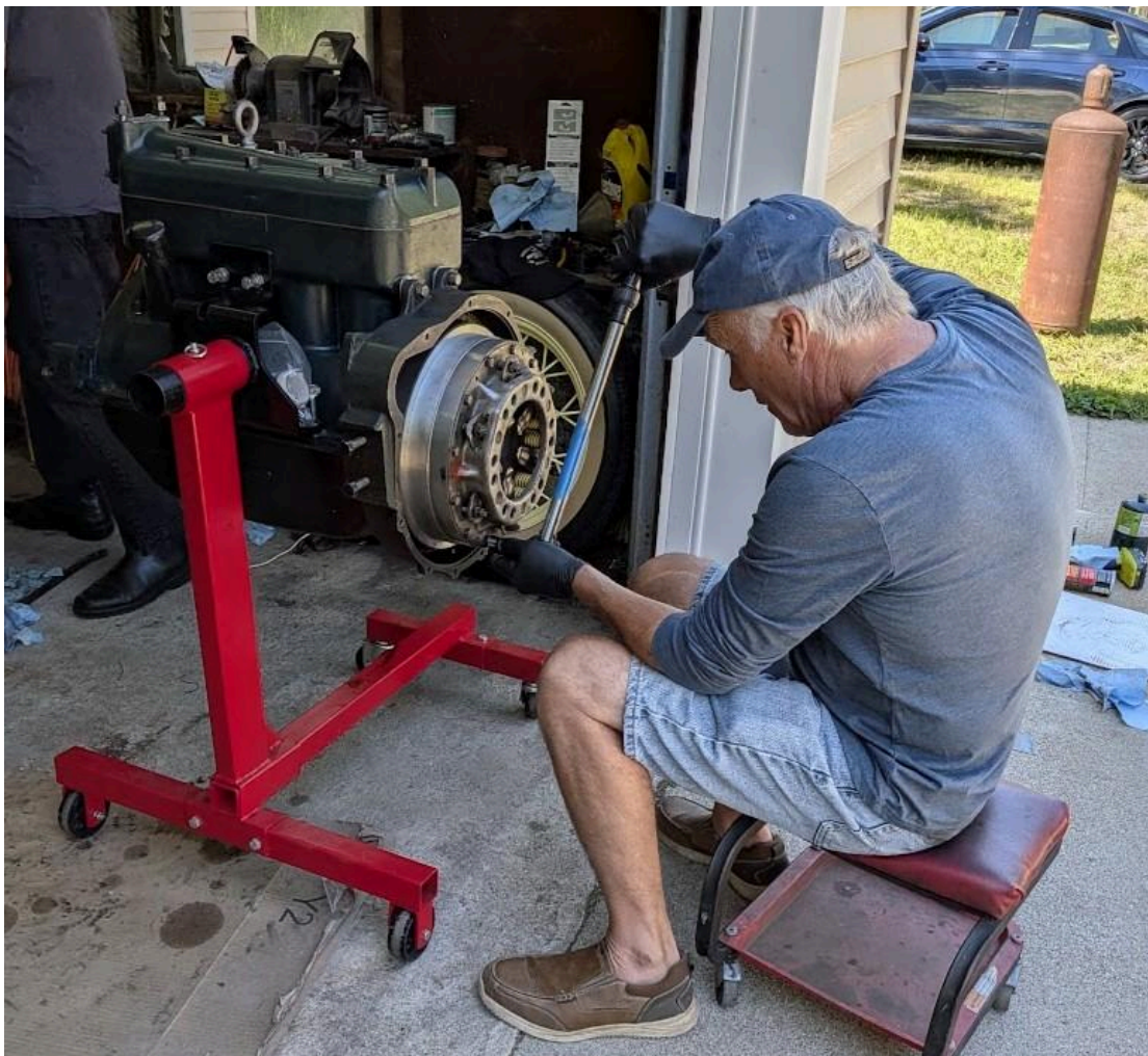
Adding the flywheel, clutch, and pressure plate to the engine
